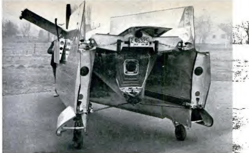
THE FLIGHT TRAILER , towed backwards on the road, is turned around on its small wheels to mate with car
